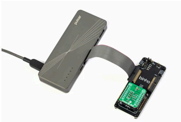
MikroBUS Adapter Board used in SPI configuration
